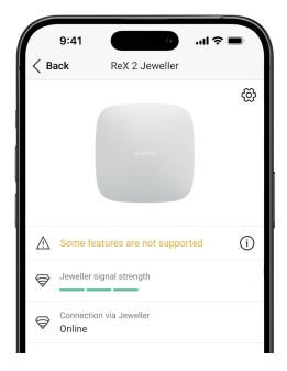
ReX 2 Jeweller can notify about malfunctions, if any. **Malfunctions** field is available in **Device States**. Clicking on (i) opens the list of all malfunctions. The field is displayed if a malfunction is detected.
