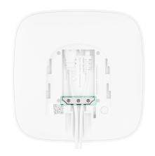
**4.** Slide ReX 2 Jeweller onto the mounting panel. After installation, check the tamper status in the Ajax app and then the quality of the panel fixation. You will receive a notification if an attempt is made to tear the range extender off the surface or remove it from the mounting panel.
