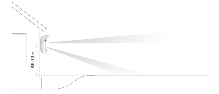
The detector should be installed on a flat, stable surface — for example, on the wall of a house or a solid fence. If the detector is installed on a shaky (unstable) surface, this will result in false alarms.
