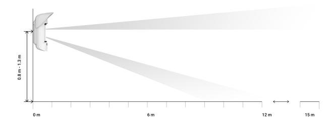
The detection distance is adjusted using the **Detection Distance** scrollbar on the rear panel of the detector. When choosing the installation location, consider the maximum detection range of the detector. It depends on the sensitivity, the position of the Detection Distance scrollbar, the type and
