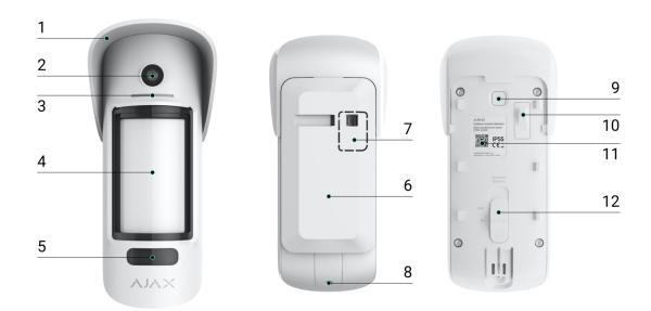
1. Hood for protecting the camera and anti-masking sensors from rain and snow.
