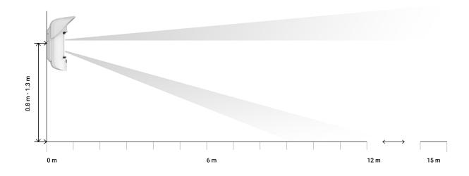
The detection distance is adjusted using the **Detection Distance** scrollbar on the rear panel of the detector. When choosing the installation location, consider the maximum detection range of the detector. It depends on the
