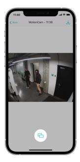
The detector has infrared backlight for shooting in the dark, which activates when there is insufficient light. Under such conditions, MotionCam takes black-and-white photos.
