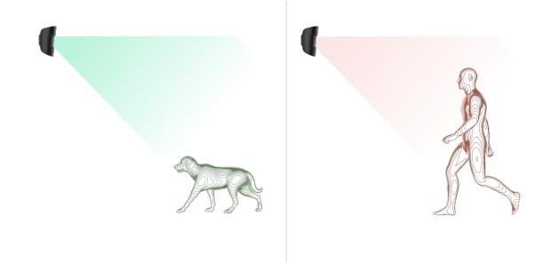
For this purpose, the detector is installed **at a height of 2.4 meters** in a place where nothing obstructs its view — for example, in a corner of a room, where the view won't be blocked by closets or other furniture. Correct setting requires the accurate choice of the detector sensitivity:
