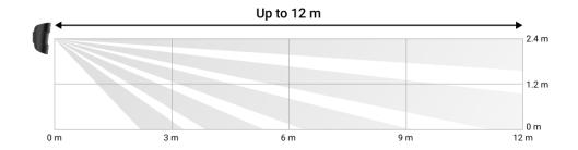
When installing the detector, run a <u>Detection Zone Test</u>. This allows you to check the operation of the device and accurately determine the sector in which the detector reacts to movement.
