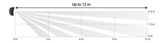
When installing the detector, perform the <u>Detection Zone Test</u>. This allows you to check the operation of the device and accurately determine the sector in which the detector registers motion.
