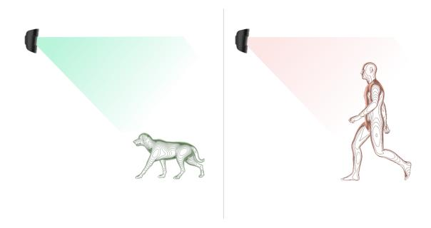
The detector is installed **at a height of 2.4 meters** without any obstruction to its view — for example, in the corner of the room, where the view won't be blocked by closets or other furniture.
